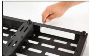
Once the tips of the screws are sticking out on the other side of the holes and the screws become easier to turn, the threads have been cut properly. Now remove the screws again.
