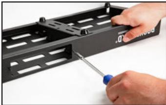
The MOD mounting screws are self-tapping, they will cut their own threads into the pre-drilled mounting holes in the RockBoard® front. Use a TX10 screwdriver to screw the mounting screws in and cut the threads. Should you do not possess a TX10 screwdriver, a wrench is included with the MOD. For the first couple
